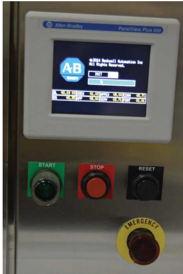
Figure 3-2: Operator Control Panel
